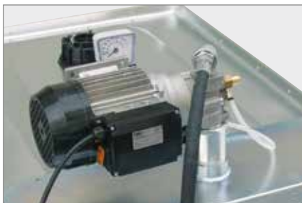
Electric pump 230 V (cannot be calibrated) with a delivery rate of 9 l/min and max. delivery pressure of 12 bar
