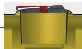
Dome with swash baffle and hinged cover
