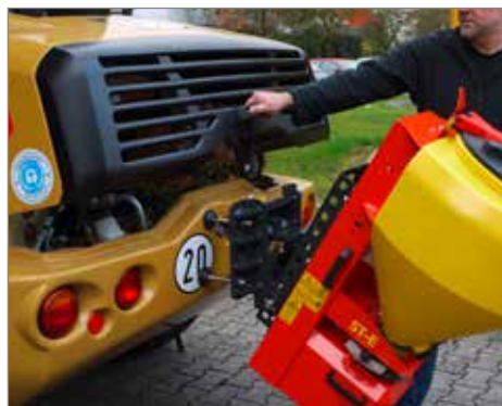
Universal holder, tiltable, as accessory (Access to motor compartment possible)
