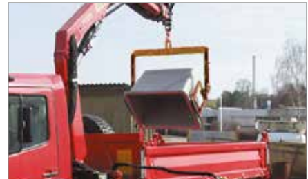
Tipping the grit out onto a truck platform (shown with 700 l the grit container)
