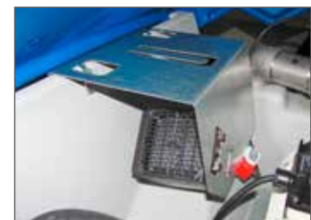
CUBE-AdBlue®-Tank, heating and thermostat
