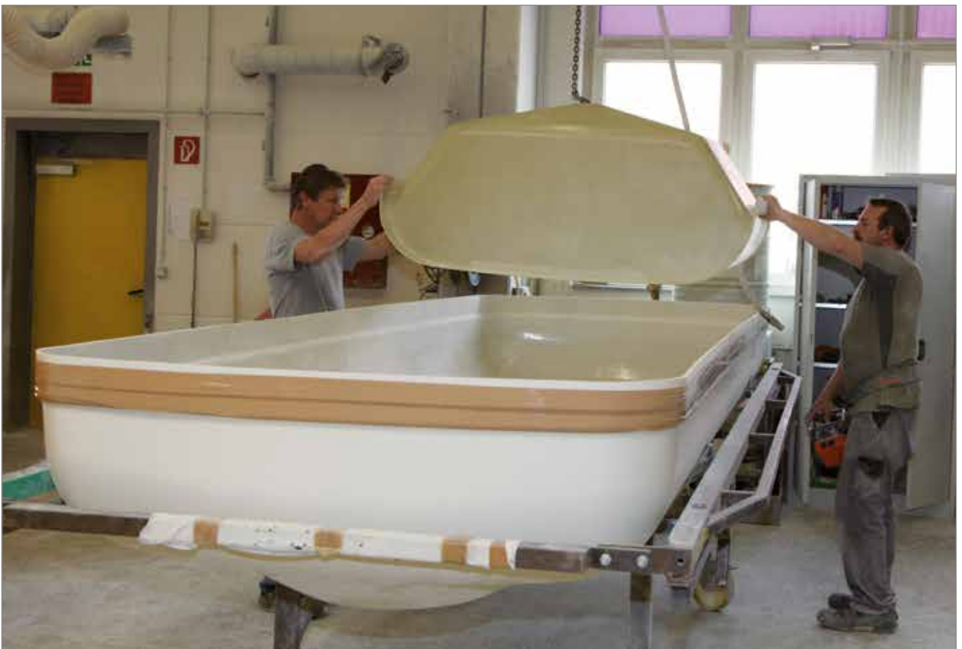
Fitting sloshing baffles in a GRP tank.
