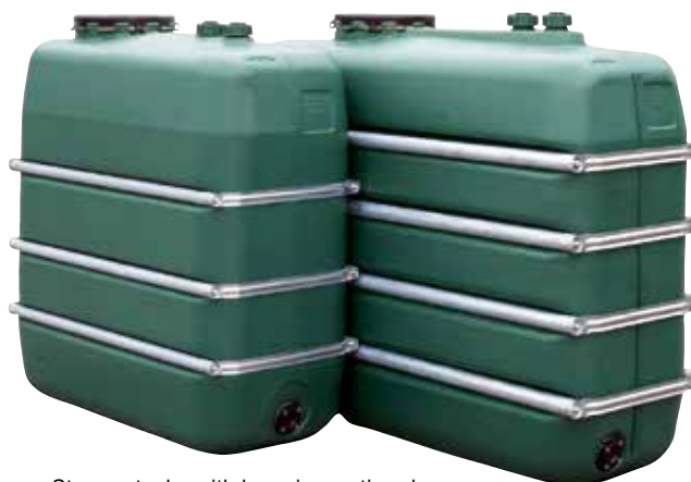
Storage tanks with large inspection dome, 2 x 2" connections and flange connection (1100, 1500 and 2000 l with bands)
