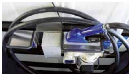
Console with pump, nozzle and hose holder
