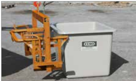
Engaging the loading frame from the side after removal of the removable lid (shown with 700 l grit container)
