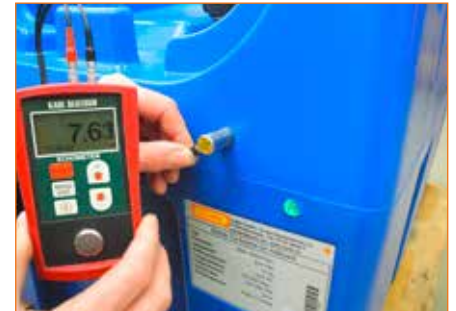
Wall thickness test on a PE tank
