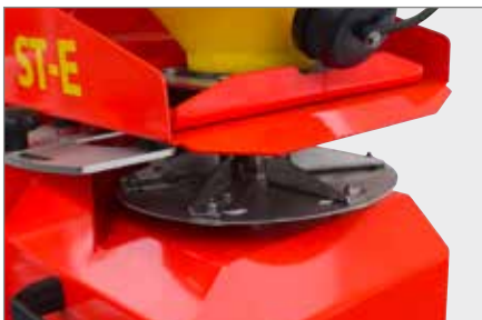
Spreader disc with central ejector shovel setting
