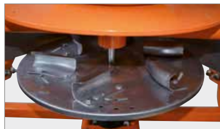
stainless steel spreader disc, adjustable
