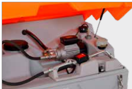
230V electric gear pump 9l/min at 12 bar with digital handheld flow meter for lubricants (cannot be calibrated)
