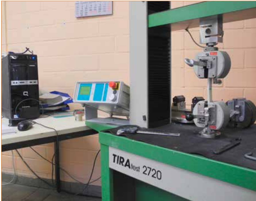
Materials testing machine for the testing of production samples
